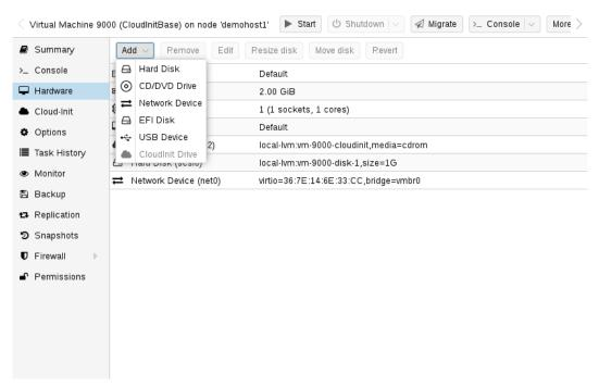
The next step is to configure a CDROM drive which will be used to pass the Cloud-Init data to the VM.
