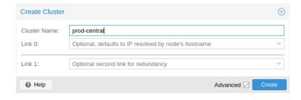
Under Datacenter o Cluster, click on **Create Cluster**. Enter the cluster name and select a network connection from the dropdown to serve as the main cluster network (Link 0). It defaults to the IP resolved via the node's hostname.
