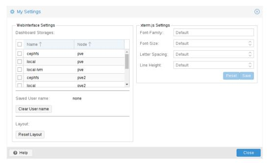
The *My Settings* window allows you to set locally stored settings. These include the *Dashboard Storages* which allow you to enable or disable specific storages to be counted towards the total amount visible in the datacenter summary. If no storage is checked the total is the sum of all storages, same as enabling every single one.
