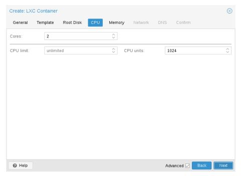
You can restrict the number of visible CPUs inside the container using the cores option. This is implemented using the Linux *cpuset* cgroup (**c**ontrol **group**). A special task inside pvestatd tries to distribute running containers among available CPUs periodically. To view the assigned CPUs run the following command:
