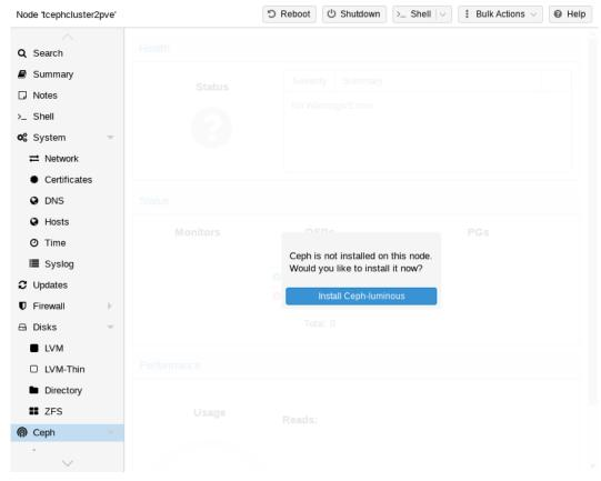
With Proxmox VE you have the benefit of an easy to use installation wizard for Ceph. Click on one of your cluster nodes and navigate to the Ceph section in the menu tree. If Ceph is not already installed you will be offered to do so now.
