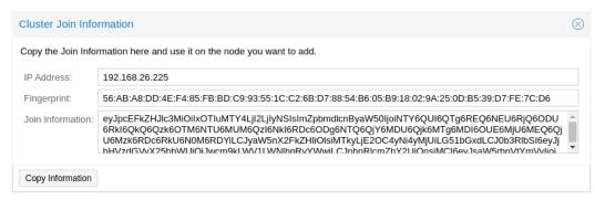
Login to the web interface on an existing cluster node. Under Datacenter o Cluster, click the button **Join Information** at the top. Then, click on the button **Copy Information**. Alternatively, copy the string from the *Information* field manually.
