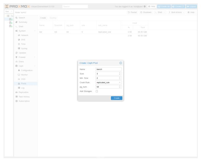
When no options are given, we set a default of 128 PGs, a size of 3 replicas and a min\_size of 2 replicas for serving objects in a degraded state.
