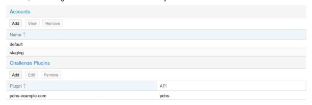
Proxmox VE supports both of those challenge types out of the box, you can configure plugins either over the web interface under Datacenter -> ACME, or using the pvenode acme plugin add command.
