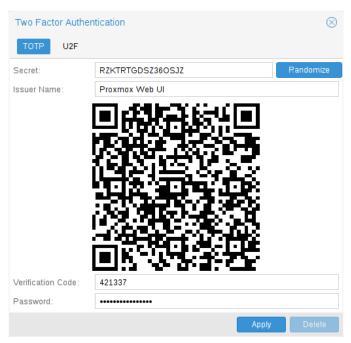
After opening the *TFA* window, the user is presented with a dialog to setup *TOTP* authentication. The *Secret* field contains the key, which can simply be generated randomly via the *Randomize* button. An optional *Issuer Name* can be added to provide information to the *TOTP* app what the key belongs to. Most *TOTP* apps will show the issuer name together with the corresponding *OTP* values. The user name is also included in the QR code for the *TOTP* app.
