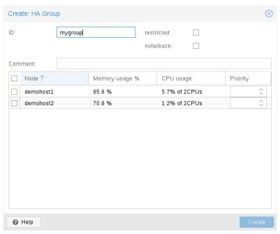
A common requirement is that a resource should run on a specific node. Usually the resource is able to run on other nodes, so you can define an unrestricted group with a single member:
