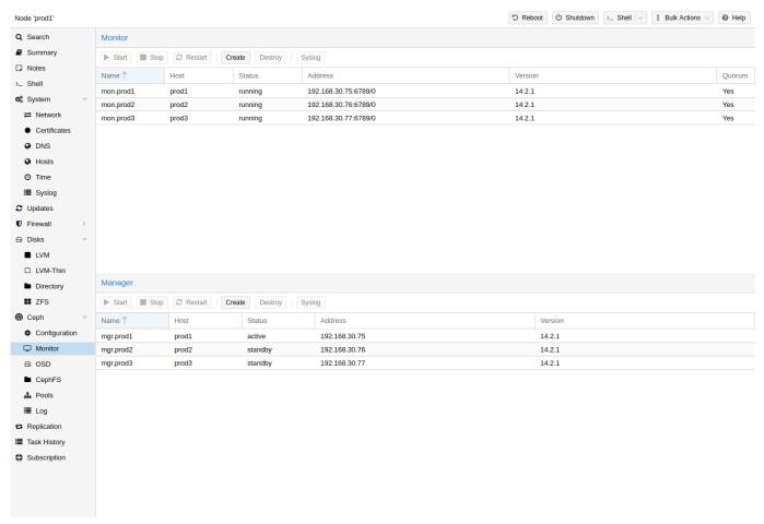
On each node where you want to place a monitor (three monitors are recommended), create it by using the  $Ceph \rightarrow Monitor$  tab in the GUI or run.
