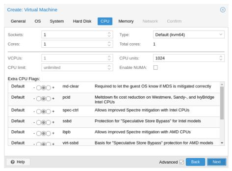
A **CPU socket** is a physical slot on a PC motherboard where you can plug a CPU. This CPU can then contain one or many **cores**, which are independent processing units. Whether you have a single CPU socket with 4 cores, or two CPU sockets with two cores is mostly irrelevant from a performance point of view. However some software licenses depend on the number of sockets a machine has, in that case it makes sense to set the number of sockets to what the license allows you.
