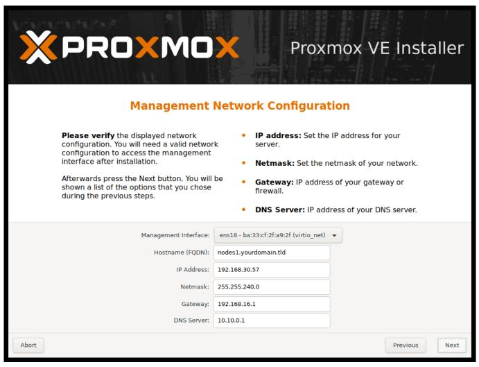
The last step is the network configuration. Please note that during installation you can either use an IPv4 or IPv6 address, but not both. To configure a dual stack node, add additional IP addresses after the installation.
