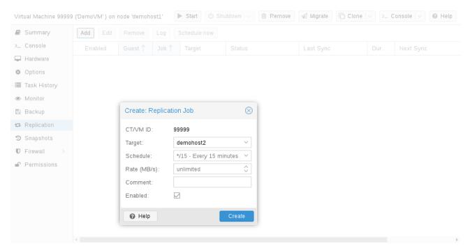
You can use the web GUI to create, modify, and remove replication jobs easily. Additionally, the command line interface (CLI) tool pvesr can be used to do this.
