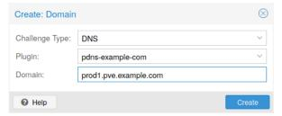
After configuring the desired domain(s) for a node and ensuring that the desired ACME account is selected, you can order your new certificate over the web-interface. On success the interface will reload after 10 seconds.
