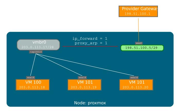
A common scenario is that you have a public IP (assume 198.51.100.5 for this example), and an additional IP block for your VMs (203.0.113.16/29). We recommend the following setup for such situations:
