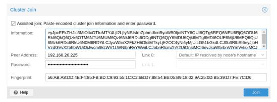
Next, login to the web interface on the node you want to add. Under Datacenter o Cluster, click on **Join Cluster**. Fill in the *Information* field with the *Join Information* text you copied earlier. Most settings required for joining the cluster will be filled out automatically. For security reasons, the cluster password has to be entered manually.
