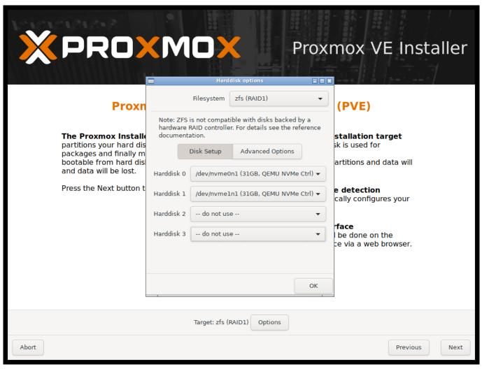
After selecting **Install Proxmox VE** and accepting the EULA, the prompt to select the target hard disk(s) will appear. The Options button opens the dialog to select the target file system.
