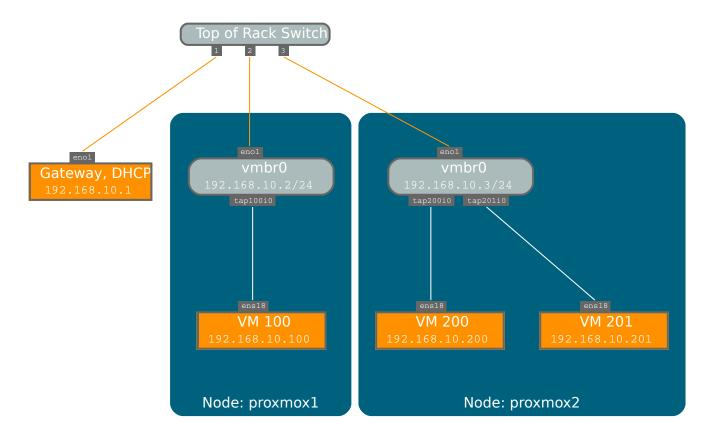
Bridges are like physical network switches implemented in software. All virtual guests can share a single bridge, or you can create multiple bridges to separate network domains. Each host can have up to 4094 bridges.
