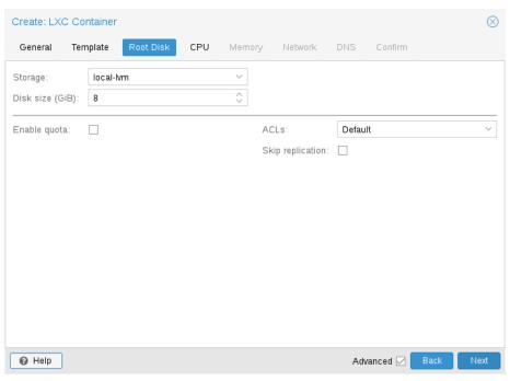
The root mount point is configured with the rootfs property. You can configure up to 256 additional mount points. The corresponding options are called mp0 to mp255. They can contain the following settings:
