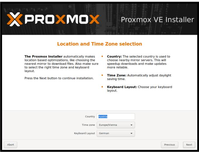
The next page asks for basic configuration options like the location, the time zone, and keyboard layout. The location is used to select a download server close by to speed up updates. The installer usually auto-detects these settings. They only need to be changed in the rare case that auto detection fails or a different keyboard layout should be used.
