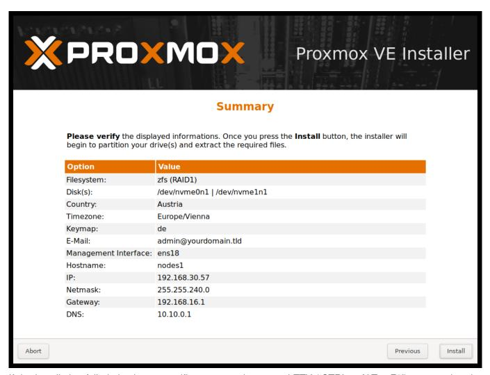
If the installation failed check out specific errors on the second TTY ('CTRL + ALT + F2'), ensure that the systems meets the minimum requirements Section 2.1.1. If the installation is still not working look at the how to get help chapter Section 1.10.
