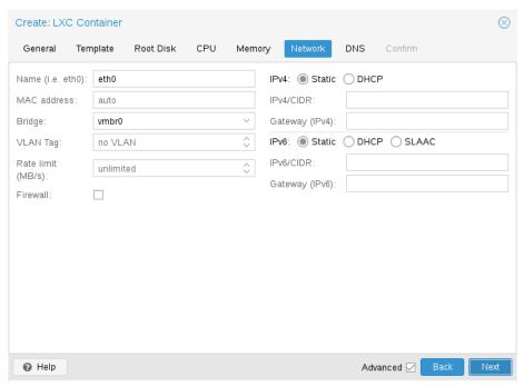
You can configure up to 10 network interfaces for a single container. The corresponding options are called net 0 to net 9, and they can contain the following setting:
