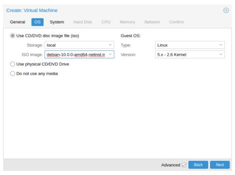
When creating a virtual machine (VM), setting the proper Operating System(OS) allows Proxmox VE to optimize some low level parameters. For instance Windows OS expect the BIOS clock to use the local time, while Unix based OS expect the BIOS clock to have the UTC time.
