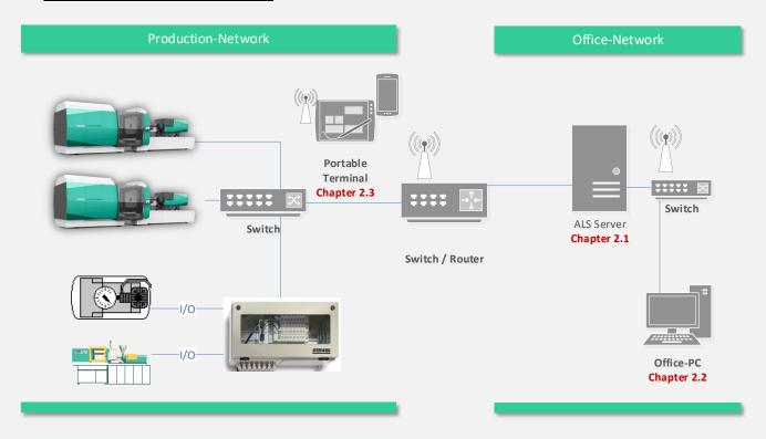
The plan illustrates the required wiring between the injection moulding machines (IMM) and the ALS Server. The wiring is to be carried out by a local IT department / company and to be adjusted to the local requirements. For the network, standard Ethernet components [100/1000BaseT(X)] are required. Configuration of injection moulding machines (IMM) is done in consultation with ARBURG.
